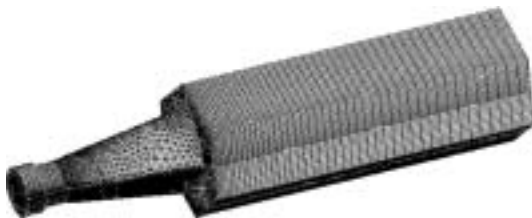
Fig. 4 Geometry and computational grids of single burner
